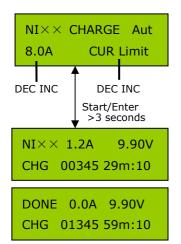
In the "Aut" mode the 1010B charges the battery at about 1C but at no more than the maximum current you set on the second line.
