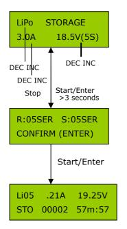
On the left side of the first line, you can set up the type of battery (LiPo, LiIo, LiFe). You can set the current and the voltage of the battery pack to be charged or discharged. The current will be used for charging or discharging the battery to reach the "storage" voltage. (Charge current: 0.05~10.0A, Voltage: 1~10 series)
