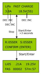
On the left side of the first line, You can set up the type of battery (LiPo, LiIo, LiFe). The values on the second line set the charge current and the voltage (cell count) of the battery pack. Press **START/ENTER** to make the value flash then press **DEC** or INC to adjust the value. After setting the current and voltage press START/ENTER again for more than 3 seconds to start the process. (Charge current: 0.05~10.0A, Voltage: 1~10 series)
