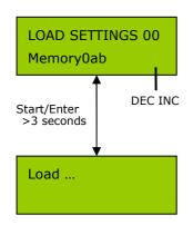
The "00" on the top line and the "memory0" on bottom line is the location you want to load dataset..
