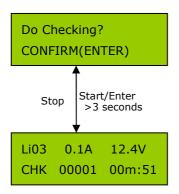
The left screen is displayed when the charger detects the battery voltage in the CHARGE or FAST CHARGE mode.
