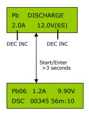
Set the discharge current and the nominal voltage of the battery. The discharge current ranges from 0.05 to 7.0A. The voltage should be matched to the nominal voltage of the battery to be discharged. The nominal voltage range is 2-36V.
