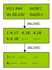
On the top line, Input voltage and Internal temperature are displayed And the bottom line, Output voltage (connected battery voltage) and external temperature are displayed
