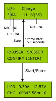
On the left side of the first line, You can set up the type of battery (LiPo, LiIo, and LiFe). The values on the second line set the charge current and the voltage (cell count) of the battery pack. Press **START/ENTER** to make the value flash then press **DEC** or **INC** to adjust the value. After setting the current and voltage press **START/ENTER** again for more than 3 seconds to start the process. (Charge current: 0.05~10.0A, Voltage: 1~10 series)
