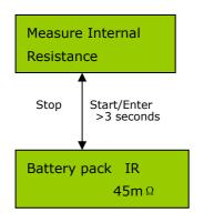
you can press **START/ENTER** for more than 3 seconds to start the process and stop at any time by **STOP**.
