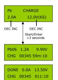
Set the charge current and the nominal voltage of the battery. The charge current range is  $0.05\sim10.0A$  and should be set to 0.1C for the battery to be charged. The voltage should be matched to the nominal voltage of the battery to be charged. The voltage parameter range is 2-36V(1-18S).
