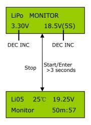
On the left side of the top line, You can set the type of battery (LiPo, LiIo, LiFe). On the second line, the cell count and the minimum cell voltage can be set. the program will monitor each cell voltage when the battery pack is discharged with external loads. The cell voltage is 3.0 to 4.2V for LiPo, 2.5 to 4.1V for LiIo, and 2.0 to 3.6V for LiFe
