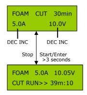
Connect the foam cutter to the DC OUT. Set up the running time, maximum current limit and the voltage. To start the foam cutter, press **START/ENTER** for more than 3 seconds. (Time is 1 to 90min, limit current is 0.05-10A, voltage is 1-40V.)
