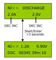
The value on the second line sets the discharge current and the terminal voltage of the battery pack.
