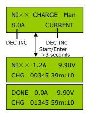
In "Man" mode the 1010B charges the battery using the current you set on the second line.
