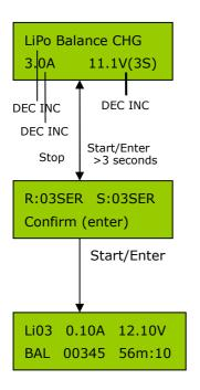
On the left side of the first line, You can set up the type of battery (LiPo, LiIo, LiFe). The values on the second line set the charge current and the voltage (cell count) of the battery pack. Press **START/ENTER** to make the value flash then press **DEC** or **INC** to adjust the value. After setting the current and voltage press **START/ENTER** again for more than 3 seconds to start the process. (Charge current: 0.05~10.0A, Voltage: 1~10 series)
