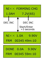
In "Forming" mode the 1010B charges the battery at up to 1C at CC/CV mode. The function is very useful for unbalanced battery pack. Forming charge will recover battery balance status.
