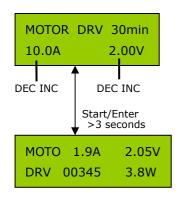
Connect the motor to the DC OUT. Set up the testing time, maximum current limit and the drive voltage. To start the motor run press **START/ENTER** for more than 3 seconds. (Time is 1 to 90min, limit current is 0.05-10A, Test voltage is 1-15V.)
