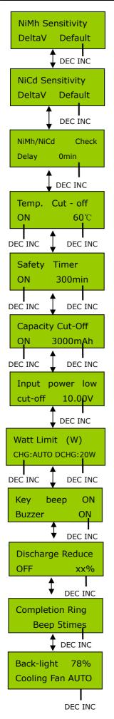
This menu shows the trigger voltage for automatic charge termination of NiMH and NiCd batteries. The effective value ranges from 1-20mv per cell. If the trigger voltage is set higher, there is a danger of overcharging the battery; if it is set lower, there is a possibility of premature termination. Please refer to the technical specification of the battery. (NiCd default: 8mv, NiMH default: 4mv)
